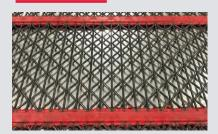
Alternating straight and formed wires vibrate at different frequencies to clean the screening surface
